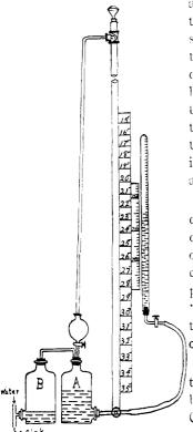
a siphon with a very short inner leg, and the long leg emptying into the sink, or as shown in the figure. To the lower part of the pipe is attached a scale, so graduated in degrees that the column of water from the bottom of the short leg of the siphon to the graduation is the calculated length for the temperature represented by the graduation. Attached to this "temperature" scale, is a sliding "pressure" sale whose divisions are r3.6 mm long.
